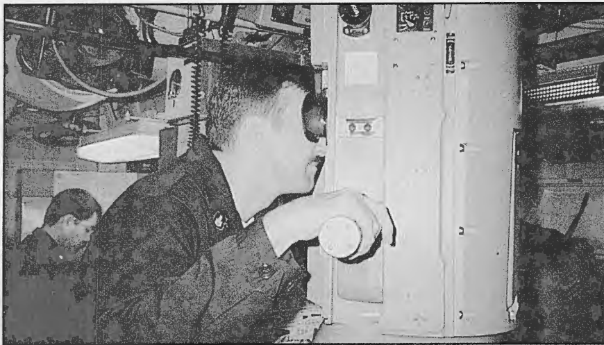
Loaded with cameras and antennas, SSN's No. 2 periscope provides visual search while sampling radio and electromagnetic environment. This scope is always manned for continuous 360-degree sweeps. Photo: Dale B. Cooper
